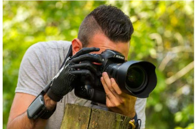
i-digits™ quantum offers compliant grip through individually powered digits with stall out ability. A manually rotating thumb in conjunction with a pulsing, enhanced grip (vari-grip), an anti-drop safety feature (auto-grasp) and the wide range of automated grip patterns lead to broad functionality.
